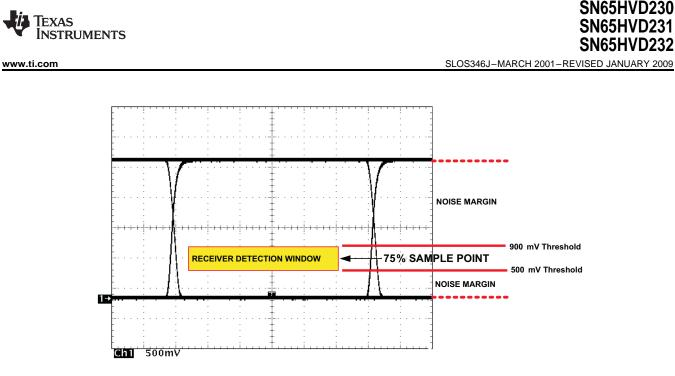
Figure 36. Typical SN65HVD230 Differential Output Voltage Waveform
