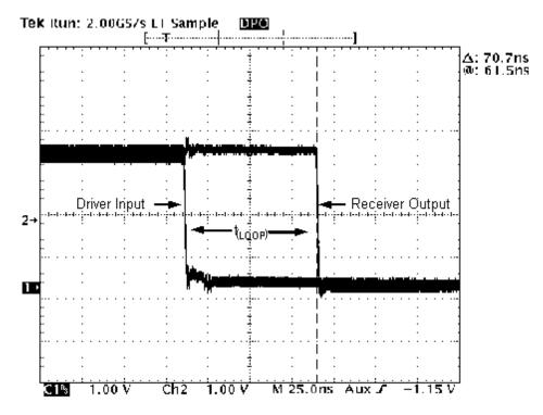
Figure 35. 70.7-ns Loop Delay Through the HVD230 With  $R_s = 0$
