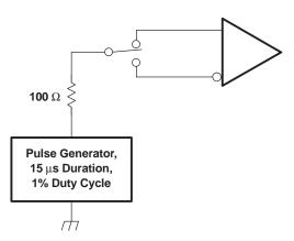
Figure 7. Overvoltage Protection
