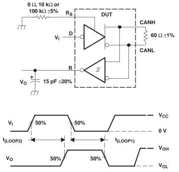
A. All V<sub>I</sub> input pulses are supplied by a generator having the following characteristics:  $t_r$  or  $t_f \le 6$  ns, Pulse Repetition Rate (PRR) = 125 kHz, 50% duty cycle.
