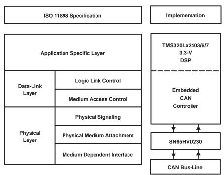
Figure 27. The Layered ISO 11898 Standard Architecture
