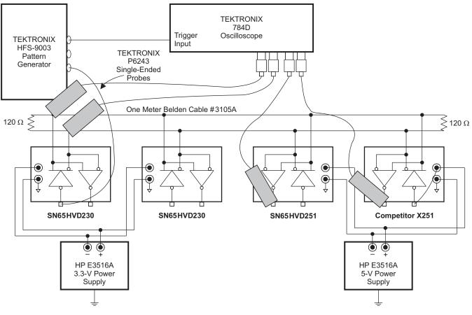
Figure 38. 3.3-V and 5-V CAN Transceiver System Testing
