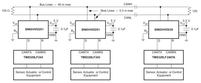
Figure 37. 3.3-V and 5-V CAN Transceiver System
