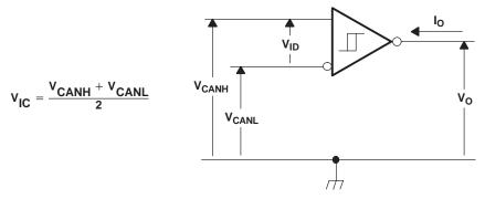
Figure 5. Receiver Voltage and Current Definitions
