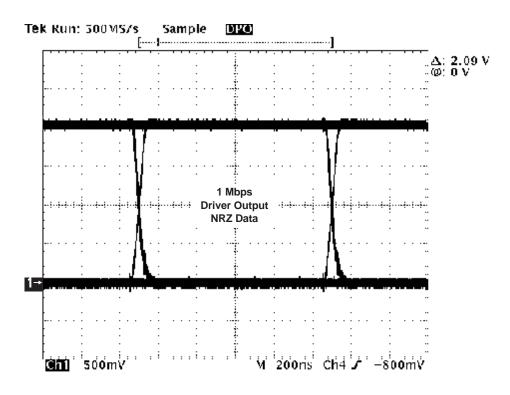
Figure 31. Typical High Speed SN65HVD230 Output Waveform Into a 60- $\Omega$  Load
